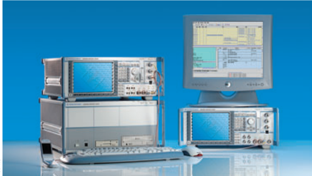
FIG 1 The new software option combines several Protocol Testers R&S CRTU to form a modular 2G/3G system simulator.
